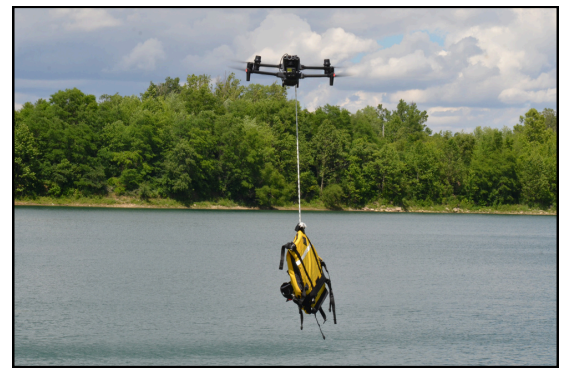
The new drone could quickly drop a flotation device to someone in the water.
