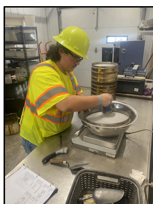
Blake Dill, a junior at Hamilton Heights High School, is pictured conducting a gradation analysis (or sieve analysis) to assess the particle size distribution as part of his internship experience this summer at E & B Paving.
